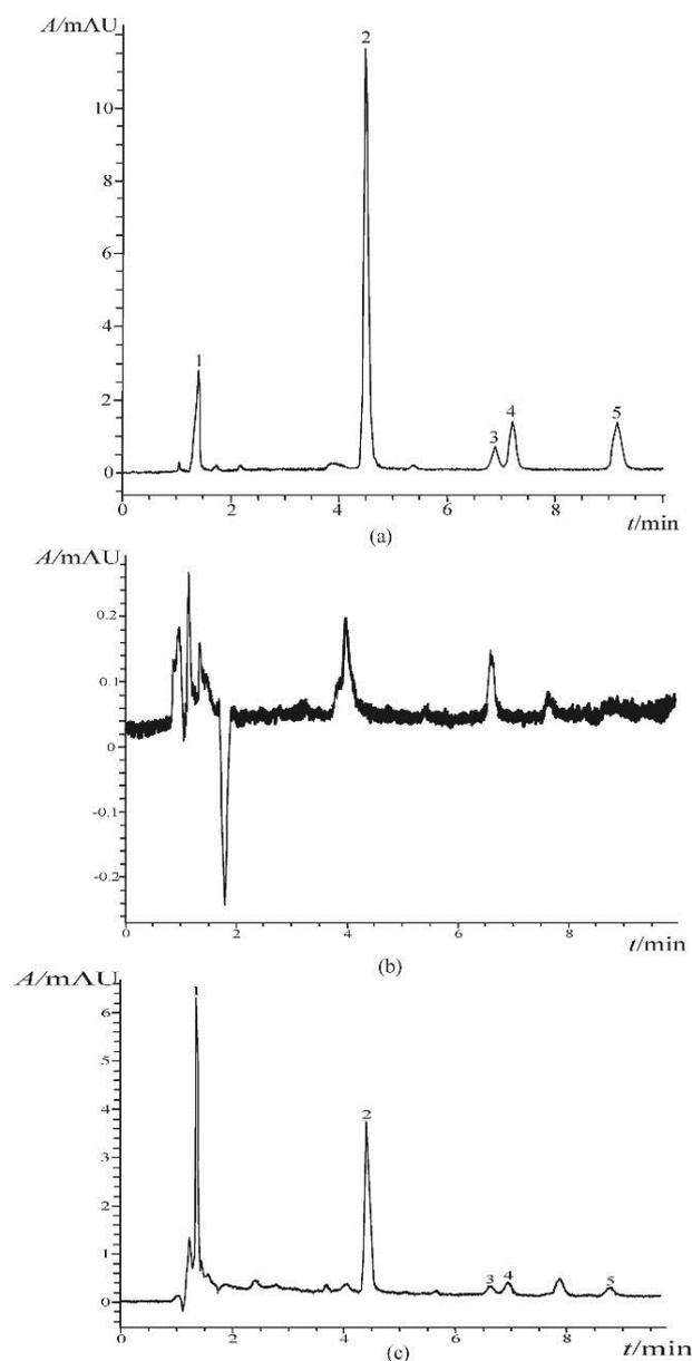
**Figure 5.** Chromatograms from standard mixture of 2,4-D (1), atrazine (2), malathion (3), fenitrothion (4) and parathion (5) at the concentrations which correspond to MRLs (a), matrix blank (b) and samples of distilled water fortified at the concentration equal to MRL for each analyte (c).
