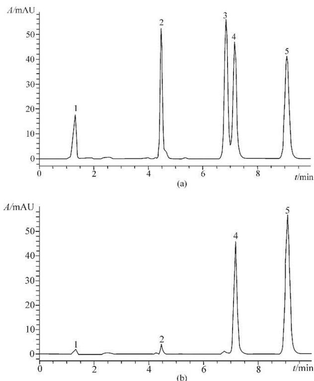
**Figure 4.** Chromatograms obtained from standard mixtures of 36.48 ng 2,4-D (1), 12.48 ng atrazine (2), 935.00 ng malathion (3), 223.68 ng fenitrothion (4) and 257.02 ng parathion (5) at 220 nm (a) and 270 nm (b) with developed method
